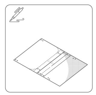
Mark the holes' location with a ballpoint pen. Don't worry about the ink, it can be removed with a cloth damped with alcohol. Mark the lines and the lower round corners for cutting.
