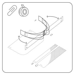
Tape the middle of strip I and 2, check the M shape the two strips made when the holes are aligned. It should be symmetrical.
