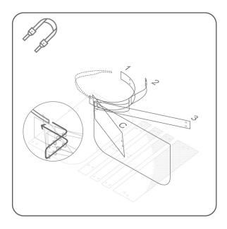
Align the holes together strips. The order from inside to outside is: 1,2,3, face-shield, and top cover. Tie the sheets with the elastic band. It should come out from upper hole and go in the lower hole.
