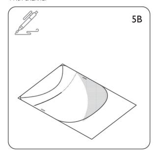
Trace the folding curves with a pen (no additional pressure is required here). If desired, fix the sheet to the template with clips or tape for more precise tracing.
