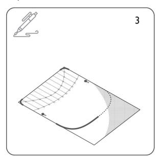
Trace out the boundary of the shield for cutting out.
