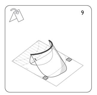
Starting on end of the crease curve, and working your way to the other end of the curve, gently pinch the sheet to fold it along the curve. If some segments do not fold easily, repeat the creasing procedure.
