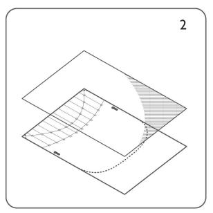
Place your transparent sheet on the template. Mark the location of the strap holes with your pen or marker. Don't worry about the ink, it can be removed with a cloth damped with alcohol.
