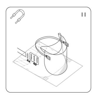
Thread the strap through the friction clips. Pass the friction clips through the holes in the shield from the back side of the shield to the front.
