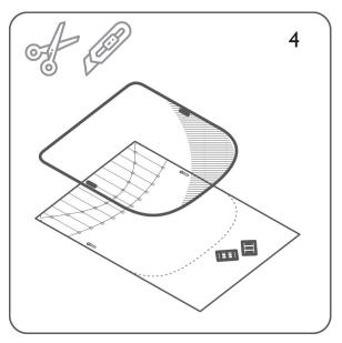
Cut the boundary shape of the shield out using scissors or a razor blade. Cut out the strap holes. You can use a hole-puncher as well to make these holes. Next, cut out the friction clips using a razor blade. Now, let's score a smile on that face!
