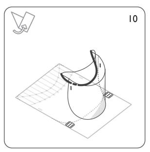
Repeat step 9 for the other curve, but this time, fold the sheet in the other direction.
