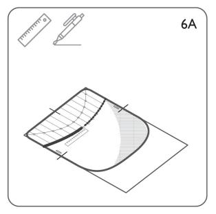
Using a ruler, and applying pressure, trace the straight segments between each consecutive point, using 2-3 strokes as needed until you see a visible indentation in the sheet.
